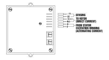
The voltage regulator also incorporates a "voltage surge protection circuit." This circuit prevents troublesome surges in the generator AC output voltage. Voltage surge is a common cause of damage to electronic equipment.
